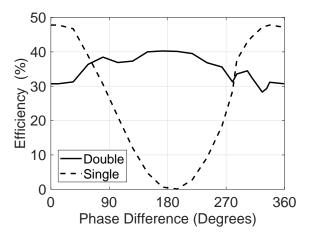
Fig. 13. Measured converter efficiency versus phase difference at the input. The input signals had frequency 2.4 GHz with  $P_{in} = 8$  dBm.
