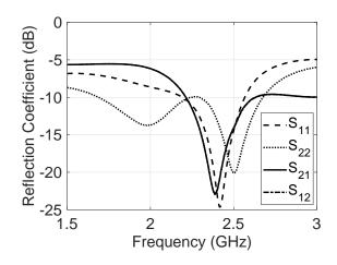
Fig. 4. S-parameters of "single" design. The VNA available input power  $(P_{\text{in,i}})$  at each port was fixed at -20 dBm.
