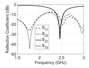
Fig. 5. S-parameters of "double" design. The VNA available input power  $(P_{\text{in},i})$  at each port was fixed at -20 dBm.
