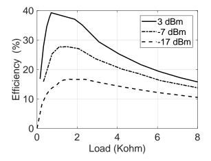
Fig. 8. Measured "double" rectifier efficiency versus load for different available input power at 2.4 GHz.
