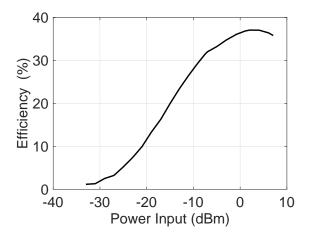
Fig. 6. Measurement rectifier efficiency of "double" design versus the available input power  $(P_{\rm in})$ . The two input signals have the same phase at the frequency of 2.4 GHz.
