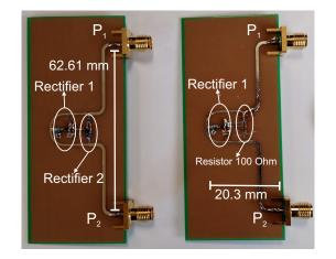
Fig. 3. The two fabricated designs on low cost FR-4 substrate. Left: The "double" design includes two rectifiers. Right: The "single" design includes one rectifier and one isolation resistor.
