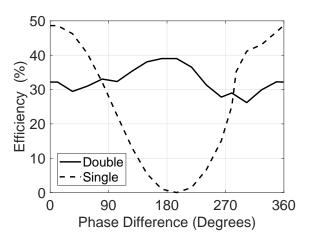
Fig. 12. Measured converter efficiency versus phase difference at the input. The input signals had frequency 2.4 GHz with  $P_{\rm in} = 3$  dBm.
