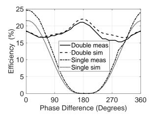
Fig. 11. Simulated and measured converter efficiency versus phase difference at the input. The input signals had frequency 2.4 GHz with  $P_{\rm in} = -17$  dBm.
