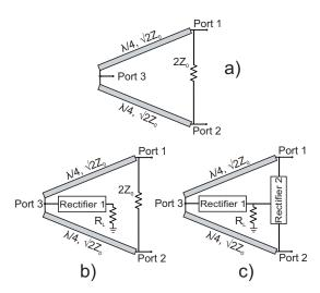
Fig. 1. Power combiner circuits with rectification capabilities. a) Typical Wilkinson combiner circuit. b) Wilkinson combiner circuit with single rectifier c) Wilkinson combiner with two rectifier circuits. One rectifier has been installed at the port 3 and the isolation resistor has been replaced with a second rectifier.
