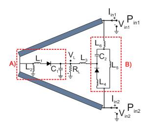
Fig. 2. Circuit of the double design. Two single rectifiers (dash rectangle) have been combined using a common load  $R_{\rm L}$ .
