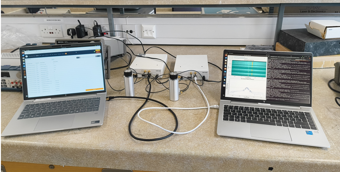
Figure 6: Laboratory Setup of Two Laptops and Two USRP N200 Radios
