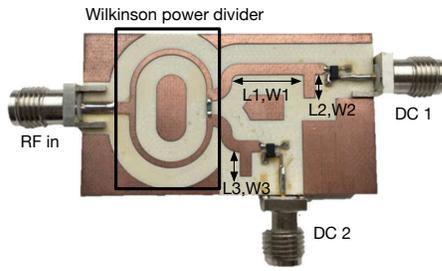
Fig. 1. Photograph of the backscatter circuit. Element values are  $L1 = 9.86$  mm,  $W1 = 1.87$  mm,  $L2 = 3.65$  mm,  $W2 = 1.87$  mm,  $L3 = 3.65$  mm,  $W3 = 1.87$  mm. Substrate for the transmission lines is Astra MT77, thickness =  $0.762$  mm,  $\epsilon_r = 3.0$ ,  $\tan \delta = 0.0017$ .
